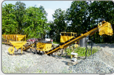
WET MIX MACADAM PLANT
