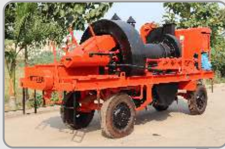
MOBILE HOT MIX PLANT
