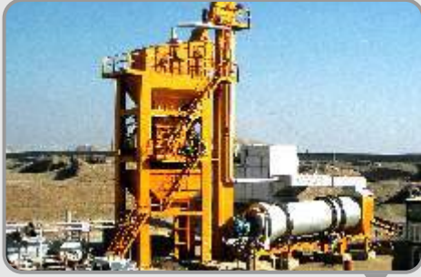
ASPHALT BATCH MIX PLANT
