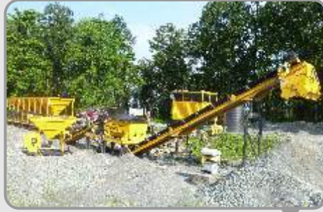
WET MIX MACADAM PLANT
