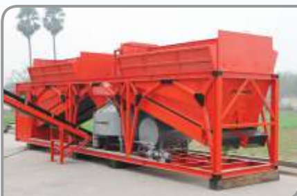
CONTAINERIZED CONCRETE PLANT
