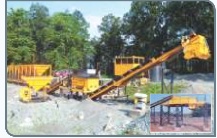
SOIL STABILISATION (WET MIX) PLANT
