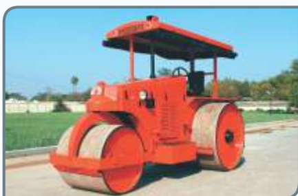
DIESEL ROAD ROLLER
