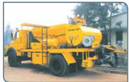
POTHOLE REPAIRING MACHINE
